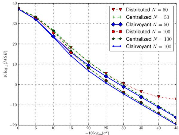
Fig. 2. MSE (dB) vs.  $-10 \log_{10} \sigma^2$  for  $N = \{50, 100\}$  and  $\delta = 0.7$ .
