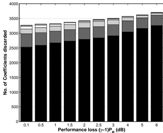
**Fig. 4.** Sparsity improvement per iteration for LP-AIC and different loss targets. Results are shown for  $N_P = 10$ .
