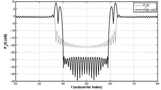
**Fig. 1.** Typical spectrum sculpting results using PSD-AIC with a target band spanning subcarriers 40 to 59.
