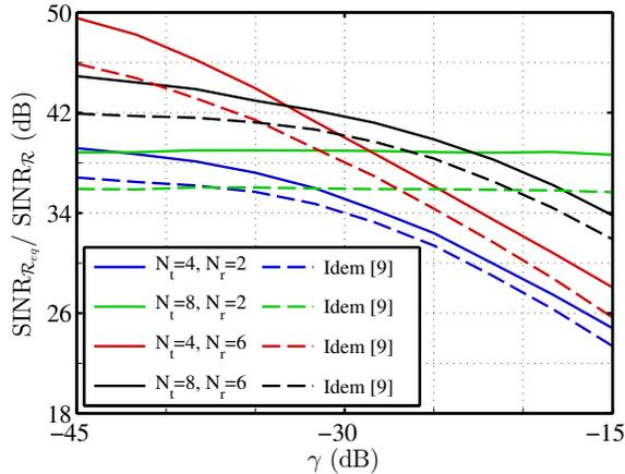
Fig. 4. SINR improvement as function of the receiver dynamic range and different relay antenna configurations.
