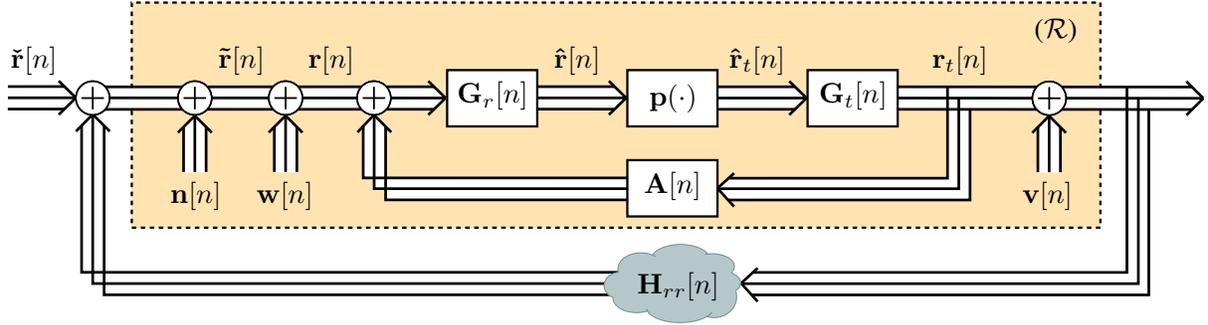
Fig. 1. System model of a relay incorporating the cancellation-suppression architecture.
