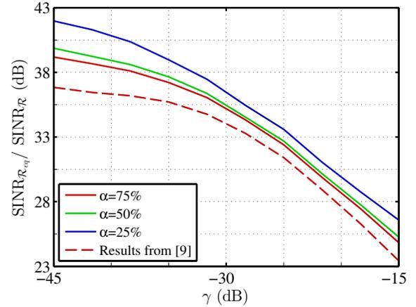
Fig. 2. SINR improvement as a function of the receiver dynamic range and different values of the power delivered at the destination.
