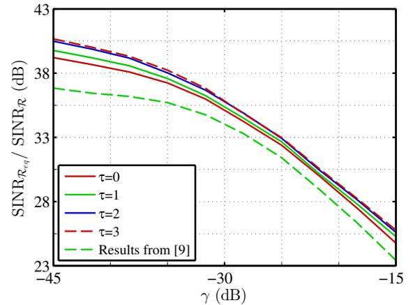
Fig. 3. SINR improvement as a function of the receiver dynamic range and different values of the effective relay-destination channel order.
