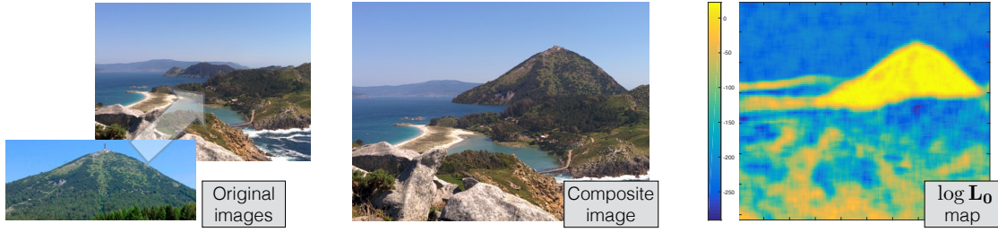
Fig. 6. A forged image is obtained by composing two JPEG images: an object from a JPEG image (downloaded from the web) has been superimposed on another JPEG background image (captured with a Nexus 5 smartphone), and the final composite image has been saved in an uncompressed format. The inserted object underwent strong modifications due to visual requirements, thus essentially losing traces of potential previous compressions, while the background image still contains those traces. The local value of \log \mathbf{L}_0 has then been computed. Overlapping windows of 120 \times 120 pixels with a stride equal to 2 pixels have been considered. The \log \mathbf{L}_0 map shows that such local analysis correctly identifies the different statistical properties within the image.
